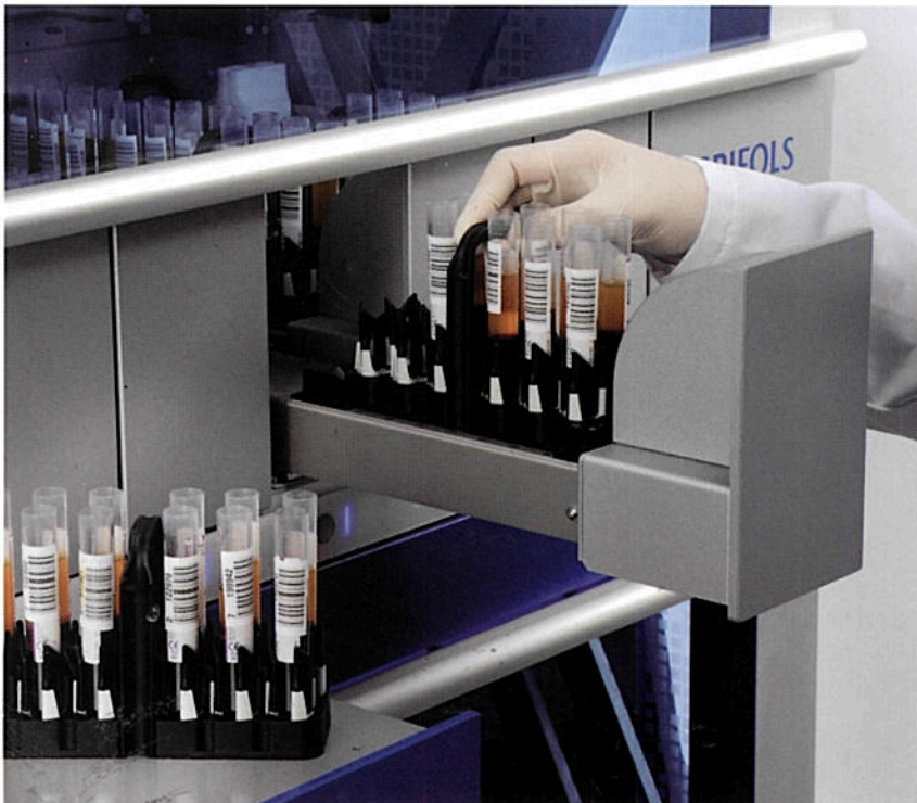
4 sample drawers with 96-sample capacity for continuous loading.
